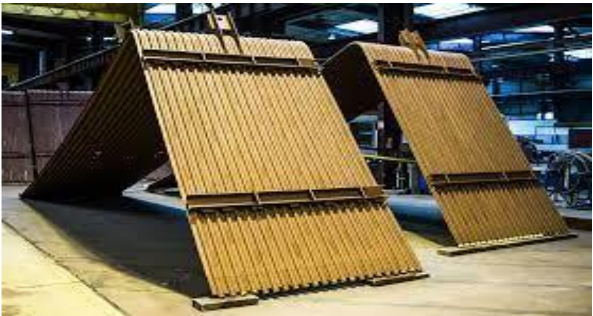
Steam boiler tube panels
